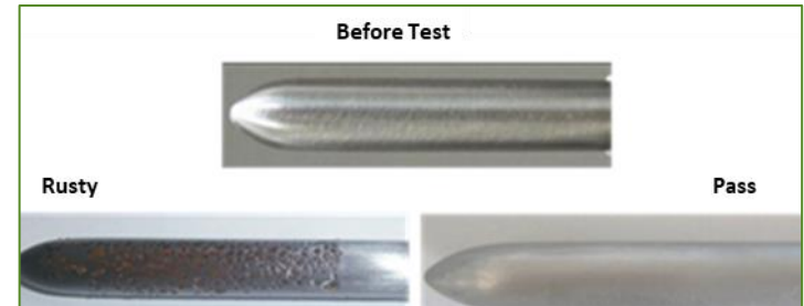
Rust test results of corrosion inhibitors.
